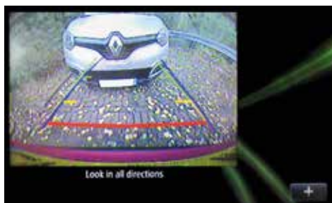
Reverse parking camera system (additional option) Reverse parking system with rear parking cameras enables you to park safely and accurately. The image is displayed in the R-link screen (when installed) with guidance aids.
