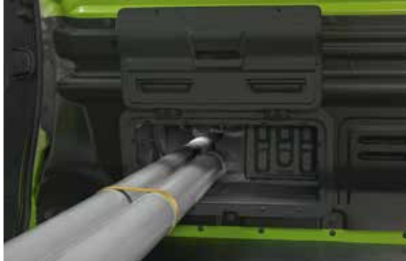
Load through bulkhead flap is magnetised to fix easily and securely in place (standard from Business+)
